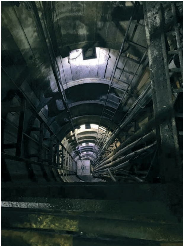
A central "lift" takes the miners and the ore carts down a shaft to different levels. (Photo: Ioannis Alexandris)
