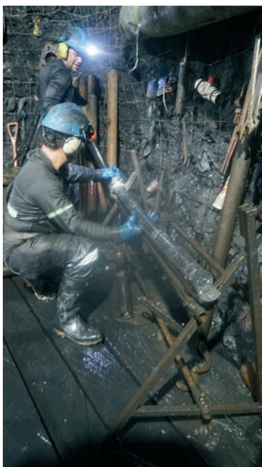
Among the modernisation efforts at Coscuez is the introduction of a diamond-drilling programme. (Photo: Fura Gems)
