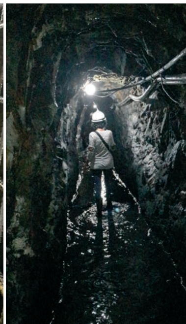
After a long staircase, we reached the main 800-metre horizontal tunnel in the Cunasa mine. Notice the water on the ground and the electrical and ventilation tubes along the wall. Water is continuously pumped out of the tunnels.
